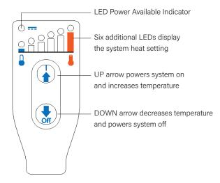
Two soft push buttons are provided for control. The rounded (convex) bump identifies the UP button, to turn on or increase the heating power. The depressed (concave) bump identifies the DOWN button, to be used to decrease the heating power, turn off the system, or cancel an alarm. A quick button press triggers a one-increment increase or decrease. Holding a button down triggers a slow auto adjustment, after a brief delay.
